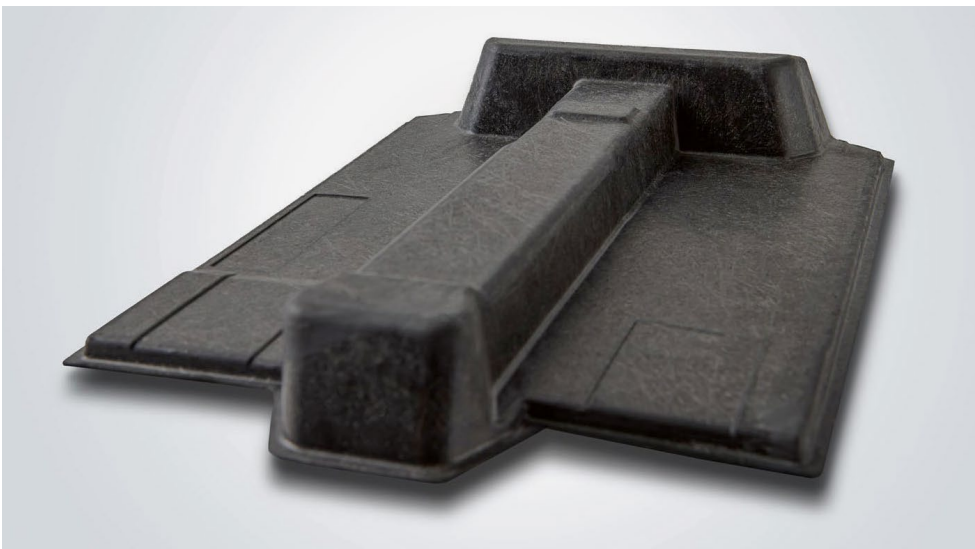
FIGURE 1 Flame protection shield demonstrator made of glass-fiber-based composite material, showing the feasibility of complex shapes (© Autoneum)
